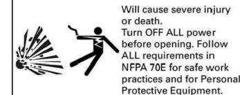
ARC FLASH HAZARD HAZARD WARNING LABELS SHALL BE FIELD MARKED/PLACED ON ALL NEW AND EXISTING ELECTRICAL DISTRIBUTION BOARDS, SWITCHBOARDS, TRANSFORMERS, PANELS, PANELBOARDS, DISCONNECTS, & MOTOR CONTROL CENTERS THAT ARE WITHIN THE SCOPE OF THIS PROJECT PER CEC 110.16. LABELS SHALL BE APPLIED TO EXISTING EQUIPMENT WHERE NEW CONNECTIONS ARE MADE. THE LABELS SHALL MEET THE REQUIREMENTS OF 110.21(B) AND ANSI Z535.4-2011 GUIDELINES BY USING EFFECTIVE COLORS, SYMBOLS OR ANY COMBINATION THEREOF.
