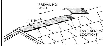
FIRST EZ-RIDGE SHINGLE COMPLETELY OVERLAPS STARTER. POSITION EACH EZ-RIDGE SHINGLE TO FOLLOW WITH AN 8 1/4" EXPOSURE BEFORE FASTFNING
