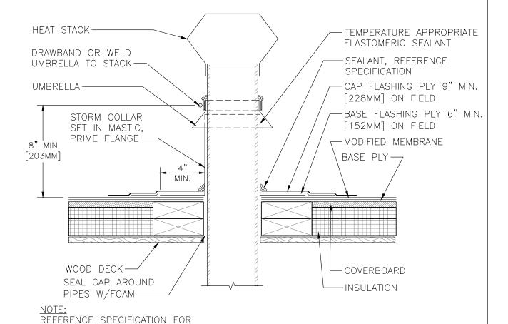
SURFACING, MEMBRANE ADHESIVE TYPE, AND INSULATION/COVER BOARD TYPE
